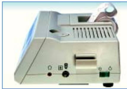
Right side with probe holder, input and output jacks, and on/off switch
